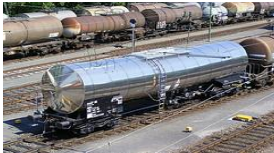
Existing 4 axle rail tank cars
