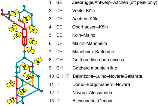
Figure 13: Missing links (numbered arrows) after realization of investment plan.
