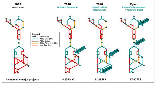
Figure 12: Development of topology for long trains with investment plan of Table 2.
