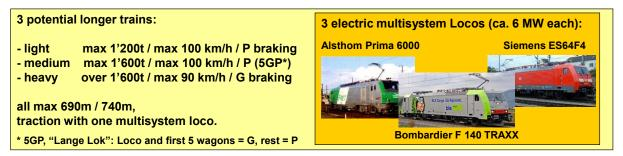
Figure 7: Combination long trains and multisystem locos.
