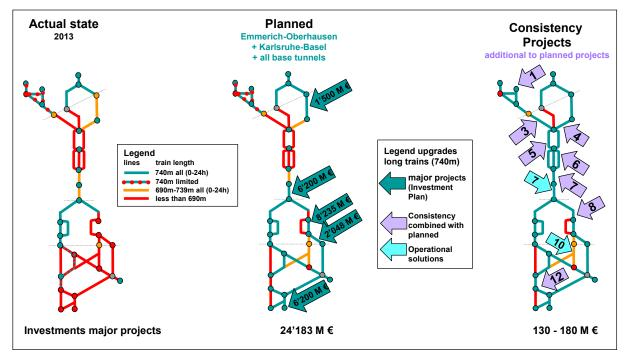
Figure 17: Development of topology for long trains with planned projects, consistency projects and operational solutions.
