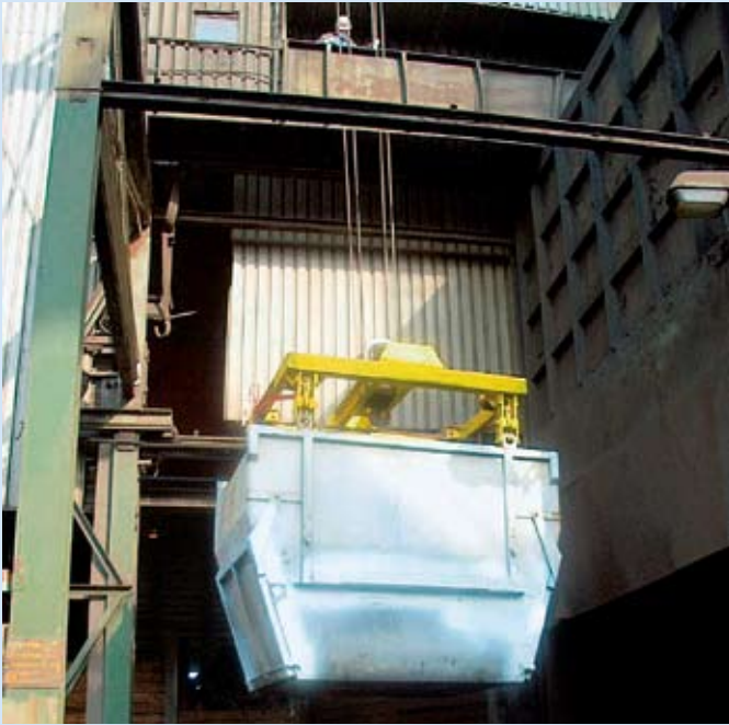
Bi-modular skips supplying the blast furnace
