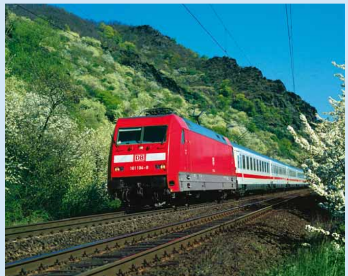
Class 101 electric locomotive of DB Fernverkehr AG: has become quieter as a result of reconstruction at a later stage.
