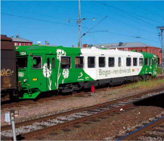
On 21 June 2005 the first train with a biogas engine was presented in Sweden - reconstructed out of a diesel train built in 1981. From September 2005 onwards it will be tested in regular passenger service between Linköping and Västervik.
