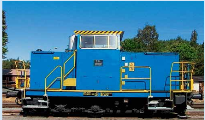
Modernised diesel locomotive belonging to Verkehrsbetriebe Peine-Salzgitter. A systematic approach has meant that noise and exhaust emissions as well as energy consumption levels have been reduced. A drip tray prevents the ground from being contaminated.
