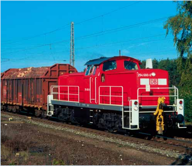
BR 294 Railion diesel locomotive (engine power class 1.000 kW). Particle and nitrogen oxide emissions have been significantly reduced by means of remotorisation.
