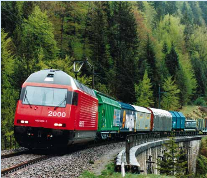
Goods waggons are deployed all over Europe. The Swiss railways are one of the pioneers of the refitting of the synthetic composite brake. This image shows a freight train with a “whispering locomotive” Re 460 (“Lok 2000”).
