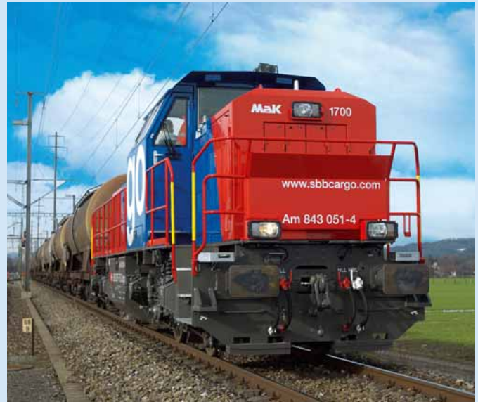
The class Am 843 belonging to the Swiss Federal Railways (SBB), the first locomotive class equipped with a particle filter as standard. Being able to operate this locomotive on tunnel tracks and construction sites, as well as inside workshops on private sidings provides the SBB with rationalisation benefits that outweigh the additional costs involved with particle filters.
