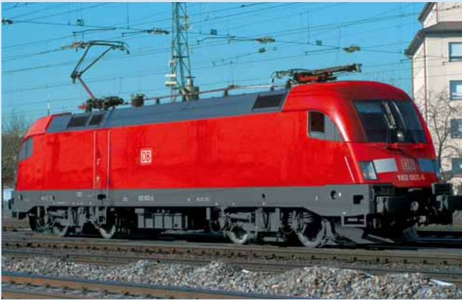
Noise reduction actively taken into consideration from the outset: Class 182. Railion ordered this class to meet the Austrian permit specifications that also stipulate noise standards. This model is now used by numerous rail companies in Germany and abroad.
